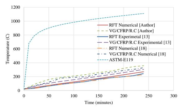
Fig. (6) Numerical results of temperature versus time compared to experimental results
