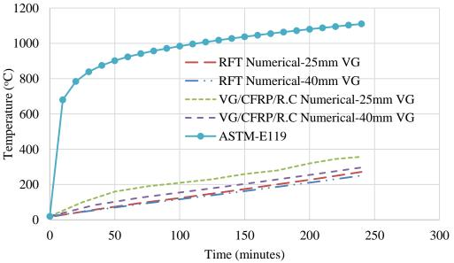
Fig. (11) Effect of changing VG thickness on thermal response of beam
