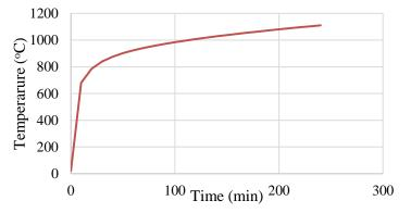
Fig. (4) Applied temperature conforming to Standard Fire Test Curve of ASTM E119
