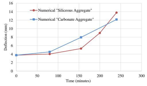
Fig. (8) Mid-span deflection for different concrete aggregate types
