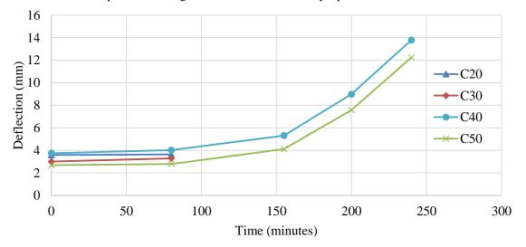
Fig. (15) Effect of changing concrete compressive strength on the structural response of beam
