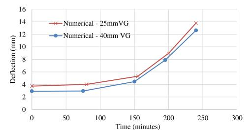
Fig. (12) Effect of changing VG thickness on structural response of beam.
