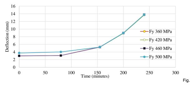
(14) Effect of changing reinforcement yield strength on structural response of beam.
