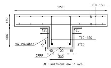
Fig. (1) Cross-section of experimentally tested T-beam [11]
