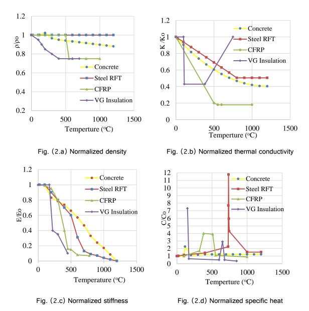
Fig. (2) Variation of mechanical and thermal properties of materials with temperature
