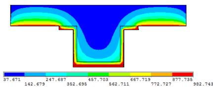
Fig.(5) Numerically predicted temperature distribution in beam cross-section (°C) after four hours
