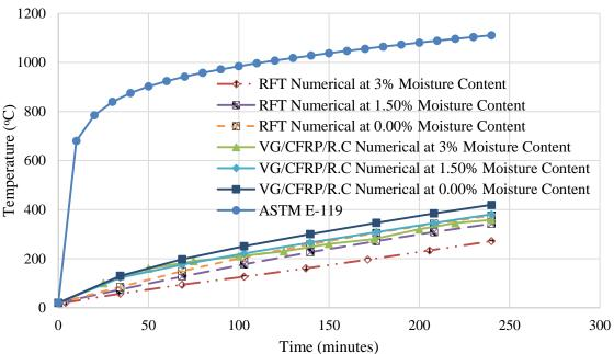
Fig. (9) Effect of moisture content on the thermal response of the beam
