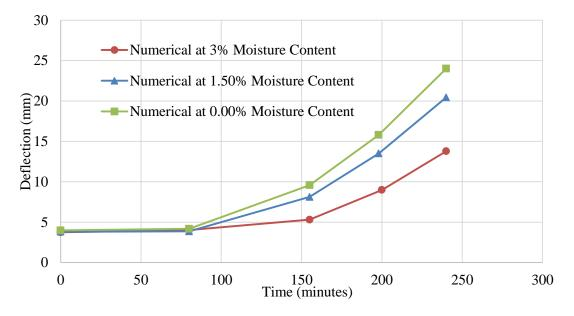
Fig. (10) Effect of moisture content on the structural response of the beam
